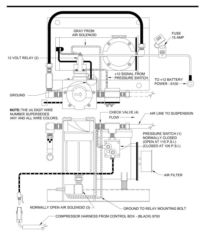
The control box sends a +12 signal to the normaly closed pressure switch (1). If the pressure is low, the 12 volt relay (2) will energize and the compressor will run. The normally open air solenoid (3) will close allowing the compressor to build pressure. When the pressure builds to 115 P.S.I. the pressure switch will open, stopping the air compressor.
