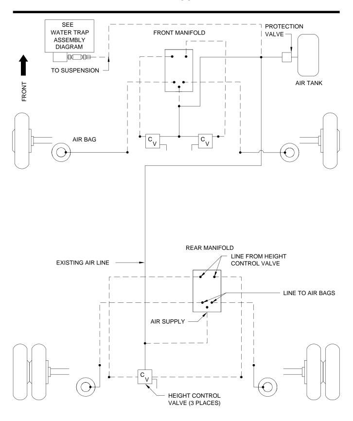
MANIFOLDS ARE MOUNTED TO MAIN CROSS MEMBERS. LEAVE AMPLE CLEARANCE FOR CONNECTION OF HOSES TO FITTINGS.
