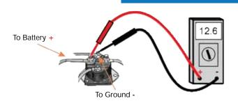
**Step 1:** Check the voltage on the battery side of the solenoid as shown on the left. The reading should be the same as the battery reading (12.6V = Full Charged Battery).
