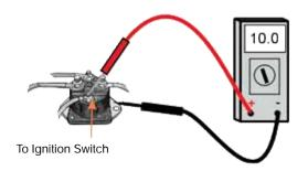
**Step 3:** Keep the negative voltmeter lead on the metal base of the solenoid and move the positive voltmeter lead to the terminal marked "S" on the solenoid. Turn the key to the start position and read the voltage. The Voltage could read a little lower than the previous reading but should never be below 10.0 volts. If the voltage is lower than 10.0 volts, You must troubleshoot the start circuit (ignition switch, voltage supply to the ignition switch, neutral safety switch).
