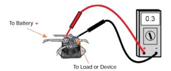
**Step 4:** Move the positive voltmeter lead to the battery terminal on the solenoid and the negative voltmeter lead to the terminal that the starter cable is attached. Activate the switch and read the voltage. The voltage should read no more than .3 volts. If the reading is more than .3 volts the contacts have excessive resistance and the solenoid be replaced.
