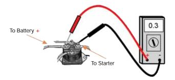
**Step 4:** Move the positive voltmeter lead to the battery terminal on the solenoid and the negative voltmeter lead to the terminal that the starter cable is attached. Turn the key to the start position and read the voltage. The voltage should read no more than .3 volts. If the reading is more than .3 volts the contacts have excessive resistance and the solenoid should be replaced.
