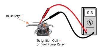
**Step 5:** Some solenoids use a relay terminal on the solenoid to power fuel pumps or supply full battery voltage to ignition coils when the starter is activated. This terminal is usually marked "I" or "R". Connect the voltmeter a shown. Turn the key to the start position. You should read no more than 0.3 volts. If you have more than 0.3 volts the solenoid should be replaced.
