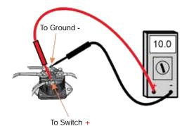
**Step 3:** Keep the negative voltmeter lead on the ground terminal of the solenoid and move the positive voltmeter lead to the terminal marked "S" on the solenoid. Activate the switch and read the voltage. The Voltage could read a little lower than the previous reading but should never be below 10.0 volts. If the voltage is lower than 10.0 volts, you must troubleshoot the switch circuit (toggle switch, push button switch, or voltage supply to these switches).
