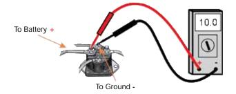
**Step 2:** With the voltmeter still connected, activate the switch and read the voltage. The voltage should not drop below 10.0 volts on this terminal. If the voltage drops below 10.0 volts, the battery cable should be cleaned or replaced. If the reading is 10.0 volts or more move on to step 3.
