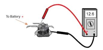
**Step 1:** Check the voltage on the battery side of the solenoid as shown on the left. The reading should be the same as the battery reading (12.6V = Full Charged Battery).
