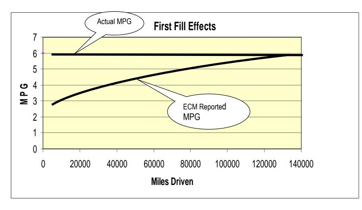
The truck has to run over 145,000 miles before the fuel ticket MPG will match the actual MPG of the truck.
