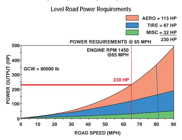
Notice that these aerodynamic treatments are more effective at higher speeds as represented by the increased vertical depth of the red graph above. Also notice that the power required to overcome things like tire rolling resistance are not affected by the aerodynamic aids.
