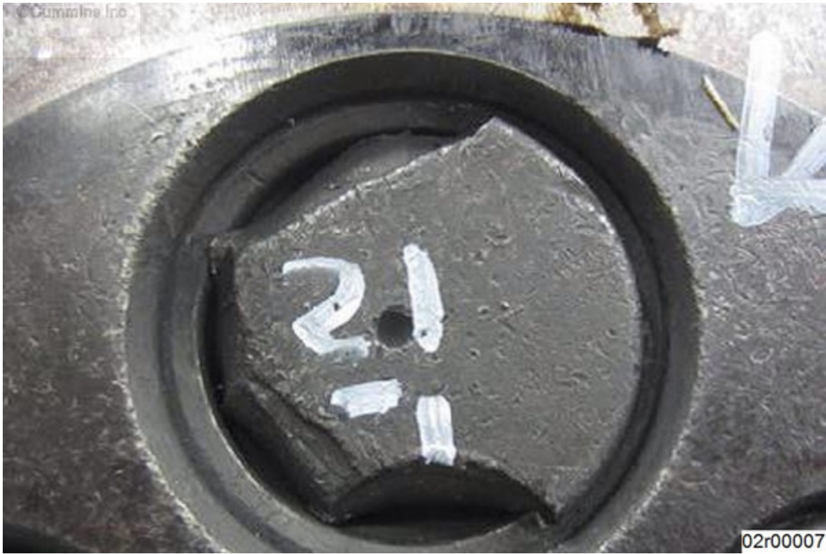
Figure 1: Broken Intake Valve in Cylinder Head
