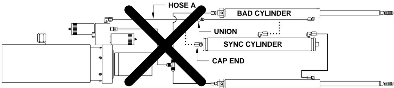
**HOSE TIGHTENING PROCEDURE:** When tightening a new hose end onto a fitting, first make the hose end snug onto the fitting with the flare of the fitting and hose end touching. Tighten the hose end 1/3 of a turn, 2 flats of the fitting. When tightening an existing hose end onto a fitting, make the hose end snug onto the fitting with the flare of the fitting and hose end touching. Tighten the hose end about 1/4 of a turn or between 1 and 1 1/2 flats of the fitting.
