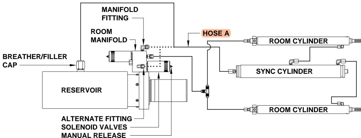
**NOTE:** On many systems, hose A goes to an alternate fitting that may be on either end of the room manifold.
