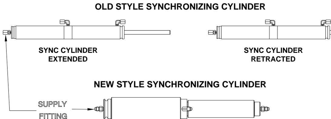
**NOTE:** The new style sync cylinder does not have a visible rod. New style sync cylinders are shipped in what would be the retracted position. For existing rooms, when the room cylinders are extended the sync cylinder will be in the retracted position.
