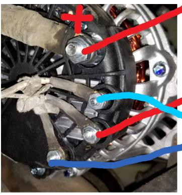
Output after install is ~14.4V DC charges house battery and Chassis battery.
