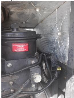
NOTE #3: Add 13 feet of #10-gauge wire to the end of the FASS fuse... and route these wires direct to the battery.
