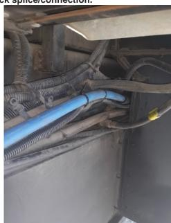
STEP #3) Route ~36' of fuel return line from the FASS pump to the fuel tank filler neck on the driver's side of the coach.
