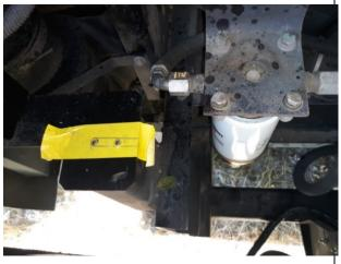
**STEP #2)** Mount the TS pump in about the same position as your primary filter (only turn it 90-degress) so you can re-use the existing fuel lines.
