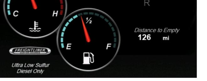
**DISTANCE TO EMPTY** IS CALCULATED BY TAKING THE FUEL IN THE TANK AND DEVIDING BY 4.3 MPG. THIS IS NOT RESETABLE
