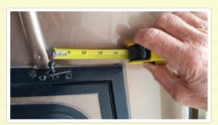
After mounting the bracket on the coach body I simply attached the gas spring, opened the door to 90 degrees, marked where that placed the door bracket, used the bracket as guide to drill three holes and mounted the bracket. When the door closes the gas spring is now collapsed almost completely. Just right. The duct tape covering the old scissor mounting hole is my temporary fix while I'm making an aluminum plate to fit.
