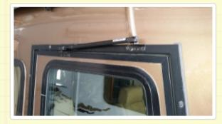
I began by drilling a third mounting hole in the bracket. The original two are probably sufficient but I subscribe to the overkill is just enough theory of engineering design.
