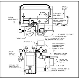
Anytime a raise function-automatic, manual up arrow or the "RAISE" button - is being used, a +12 volt signal is sent to the compressor from the control box. This turns a single output compressor on if air pressure in the system is below approximately 105 psi. A +12 volt signal from the control box will turn a two output compressor on at anytime. A +12 volt signal through the auxillary pressure switch for auxillary air will turn the compressor on if system air pressure drops below 60 psi.
