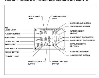
All HWH air leveling touch panels have the same buttons and indicator lights. However, it is important to note that some of the buttons and lights react differently with different systems.
