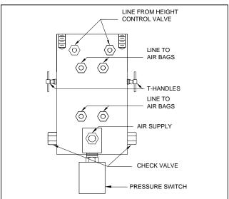
The manifold with two pressure switches monitors air pressure in the air bags. The single pressure switch on a manifold monitors system air pressure.
