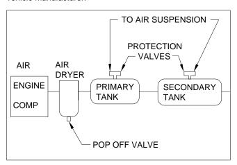
Although it may vary between different vehicles, it normally takes at least 60 psi to start lifting a vehicle. Most vehicles will require 90 psi to obtain maximum lift. Some may require up to 130 psi to obtain maximum lift.
