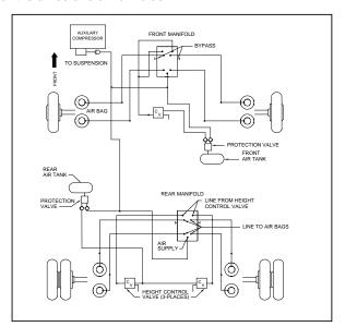
The next two diagrams show two different air compressor arrangements. The first compressor only has one air outlet. It should only be used to supply air for the leveling system. The second air compressor has two outlets, one is for the leveling system and the other supplies air to the main vehicle air system.
