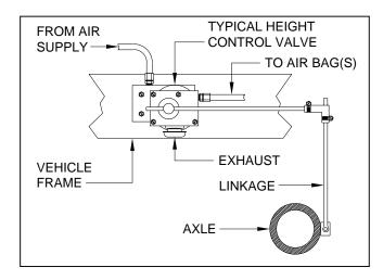
There can be different height control valve arrangements. There can be one valve for the front axle and two valves for the rear. That can be reversed having two valves on the front axle and one valve on the rear. There can also be different air bag arrangements. There can be one or two air bags for each wheel. Sometimes, the front axle will be different than the rear axle.
