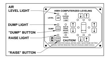
Momentary "DUMP" and "RAISE" buttons. If the system has momentary "DUMP" and "RAISE" buttons, the buttons can be used about anytime. The ignition can be on or off. The park brake does not have to be set. The touch panel can be on or off. The only time the "DUMP" and "RAISE" buttons will not work is if the touch panel is in the automatic leveling or SLEEP mode.
