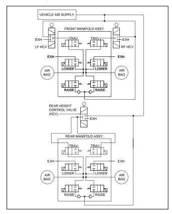
Note that there are three valves for each air bag. There is a raise valve, a lower valve, and a travel valve. The valves are very simple, electronically operated valves. All of the valves are normally closed valves, which means that they will not let the air by until they are electronically activated. Each valve has an electronic coil which is activated by applying (+12) volts to one side of the coil and grounding to the other side of the coil.
