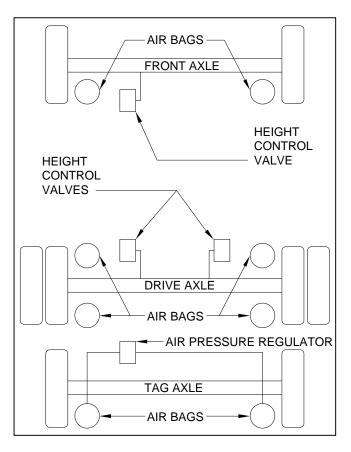
All of these different situations must be considered when designing an air leveling system for a vehicle. The HWH air leveling system works in conjunction with the vehicle suspension not only for leveling but also when the vehicle is in the travel mode.
