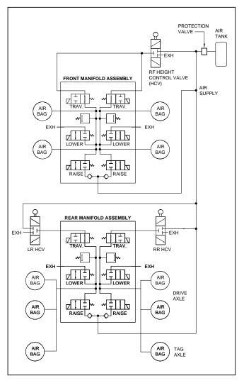
When the leveling system is in the travel mode the tag axle is allowed to function as it normally would.
