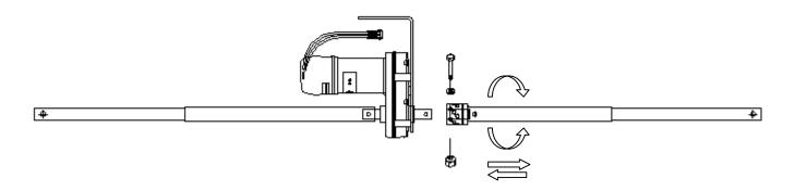
With room about half way out, release slide-out motor brake.
