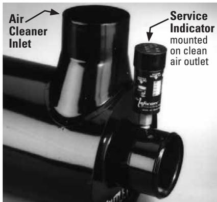
Filter service indicators are very effective when mounted on the outlet tube of the air cleaner, see The Informer™ above. This gives the operator constant and accurate visibility of filter life.
