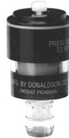
Through the clear window, a green flag shows when air filter restriction is below the service point. When the restriction reaches its limits, an orange flag imprinted with "change filter" pops up.
