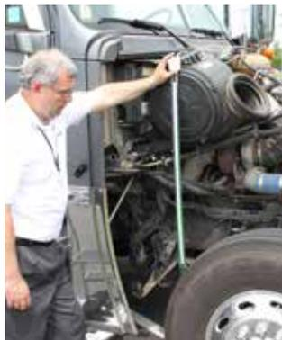
Magnets conveniently hold top and bottom ends of manometer to side of equipment or vehicle. Special shut-off valve eliminates the need to empty water after use.
