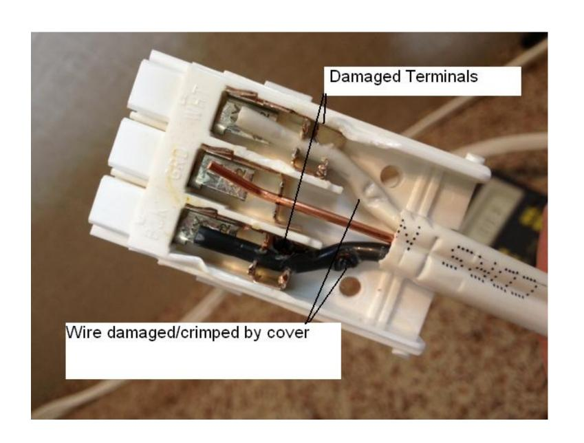
Mounting screw was driven through the white conductor creating an intermittent connection and a potentially dangerous condition
