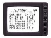
Press the <u>VIEW</u> key on the keypad. The "TODAY" screen will display on the backup monitor.
