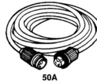
In some hook-ups the power cord may not be long enough and extension cords are required. ALWAYS use a cord with the gauge of wire equal to or greater than the power cord. Should you use a cord with a smaller wire, overheating, loss of amperage, and possible melting could occur.
