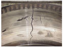
Excessive drum crack
