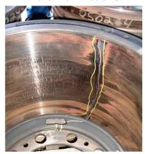
Cracked brake drum
