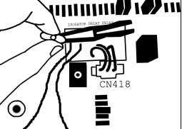
Set mounting hardware aside as it will be needed during reinstallation.
