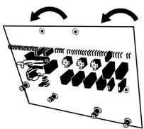
Connect one BLUE wire to 12-Volt House Non-Switch bolt (J2) and remaining BLUE wire to 12-Volt Battery Chassis bolt (J3)
