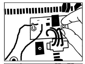
Locate the House Power Distribution Panel and remove mounting bolts as indicated.
