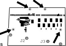
Secure fuse extractor to longer mounting stud. Insert connector into jack CN418.
