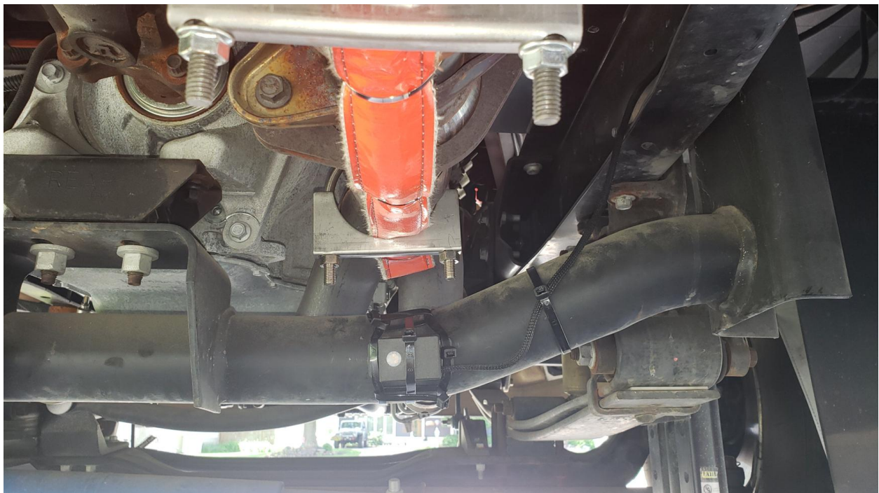
Picture of the motion sensor installation on the tubular crossmember
