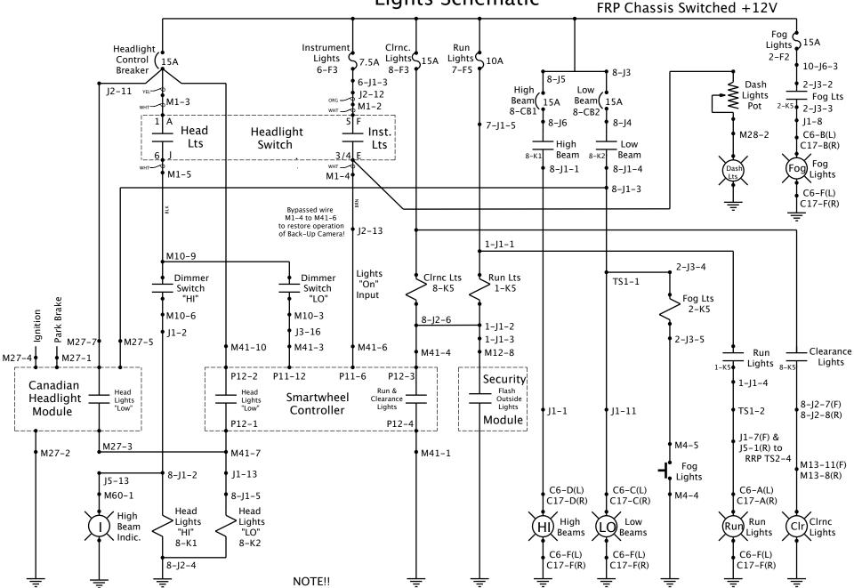
There are at least two missing connections. There has to be connection to the dash module that tells it the headlights are "ON", in the "Headlights" position. And, there has to be a connection that needs to come from M28-2, that "wakes" the dash when the instrument lights are in other than the "OFF" position. Both are true, because the light switch makes the dash come alive in both "Run" and "Headlights" position, and the dash action is different, in the two switch positions.
