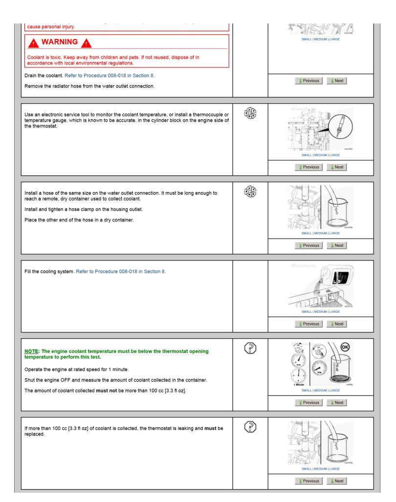
Complete the following test in-chassis to determine the thermostat opening temperature.
