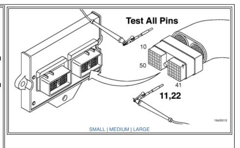
Measure the resistance from pin 22 of the engine harness to engine block ground.
